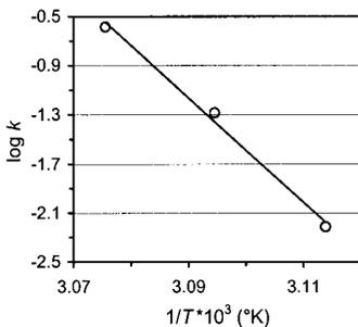
Fig. 3. Arrhenius plot for temperature effects on thermal death rates for older red flour beetle larvae. Line represents linear regression equation  $\log k = 130.21 - 42.52 \cdot 1000/T$  ( $r^2 = 0.99$ ) where  $k$  is thermal death rate constant and  $T$  is temperature.
