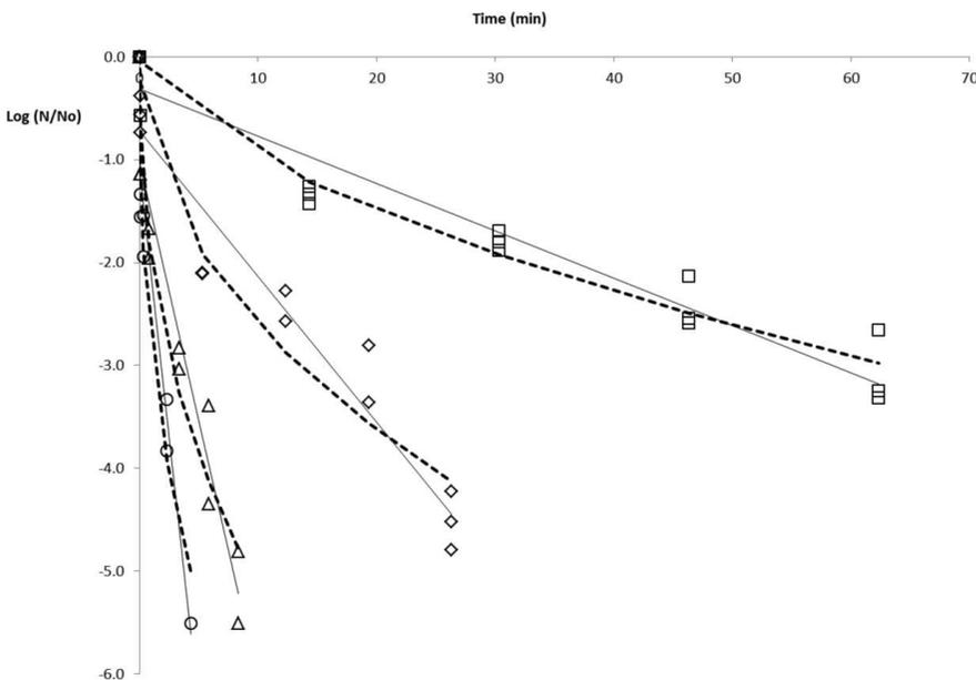
FIGURE 1. Heat inactivation kinetics of *Salmonella Enteritidis* PT 30 inoculated in almond kernel flour with an  $a_w$  of 0.888 at different temperatures ( $\circ$ , 68°C;  $\triangle$ , 65°C;  $\diamond$ , 62°C;  $\square$ , 59°C). — and --- lines are the fits of the primary models: the first-order kinetic model and modified Weibull distribution, respectively.
