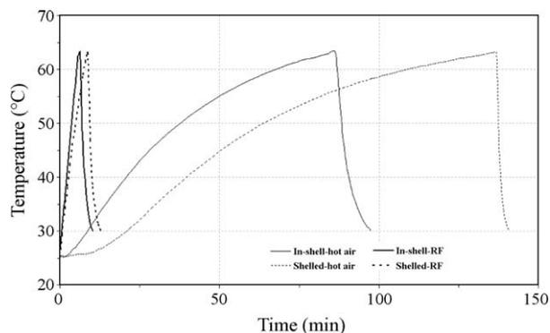
**Fig. 4.** Typical temperature–time histories of in-shell and shelled almonds in the center of a 10 cm thick container in hot air heating at 63 °C as compared with stationary hot air assisted RF heating of shelled (gap = 11 cm) and in-shell (gap = 12 cm) almonds followed by forced room air cooling in single layer samples.
