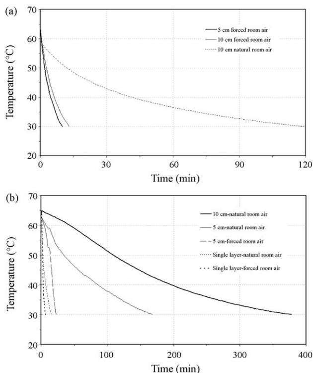
**Fig. 3.** Cooling curves of in-shell (a) and shelled (b) almonds in the sample center as a function of sample thickness under natural and forced room air cooling.
