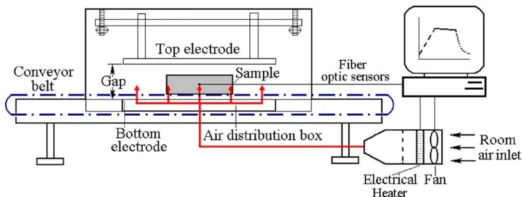
**Fig. 1.** Schematic view of the pilot-scale 6 kW, 27.12 MHz radio frequency (RF) unit showing the two-pair plate electrodes, conveyor belt and the hot air system (Wang et al., 2010).
