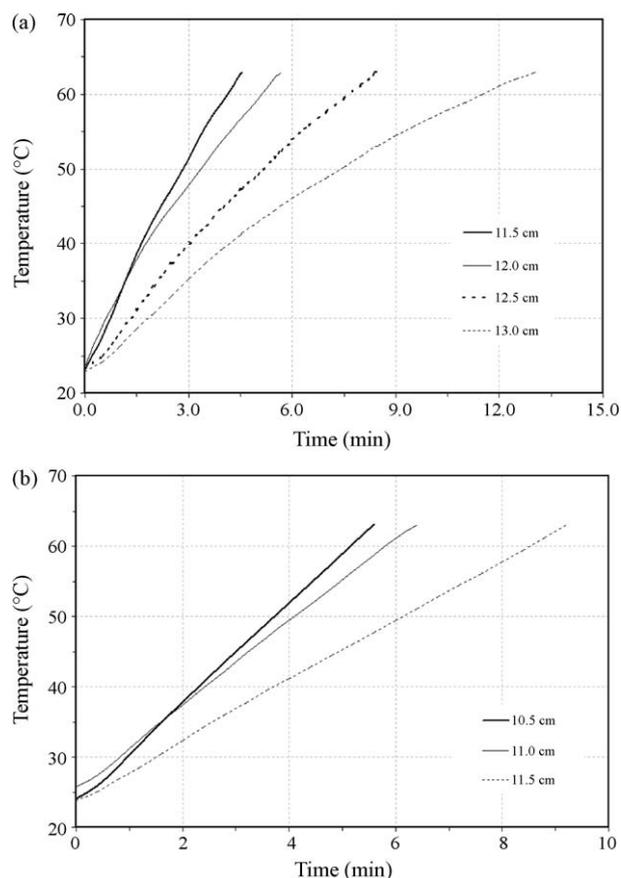
**Fig. 2.** Temperature–time histories of the RF heated in-shell (a) and shelled (b) almonds in the center of the 10-cm thick container as a function of the electrode gap without movement, hot air heating, and mixing.
