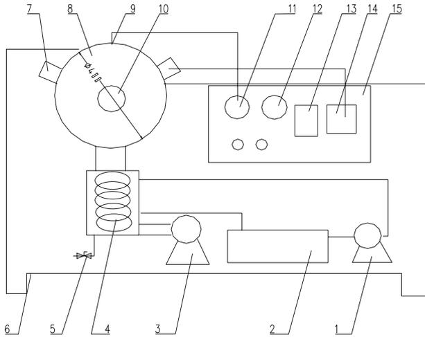
**Figure 2** Schematic of the microwave freeze dryer. 1. refrigerator 2. cooler 3. vacuum pump 4. cold trap 5. blowdown valve 6. equipment support 7. magnetron 8. drying cavity 9. infrared thermoscope 10. observation window 11. thermometer 12. pressure detector 13. PLC controller 14. power regulator 15. control box.
