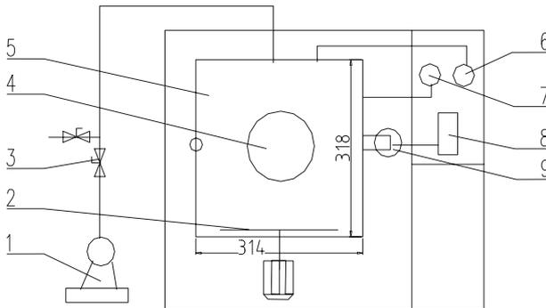
**Figure 3** Schematic of the microwave vacuum dryer. 1. vacuum pump 2. rotating tray 3. valve 4. observation window 5. drying chamber 6. infrared thermometer 7. vacuum gauge 8. magnetron power control unit 9. magnetron.
