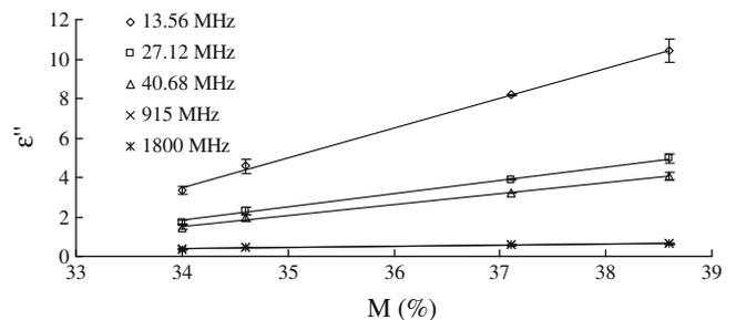
**Fig. 7.** Moisture content dependency of bread loss factor at five frequencies and 25 °C.
