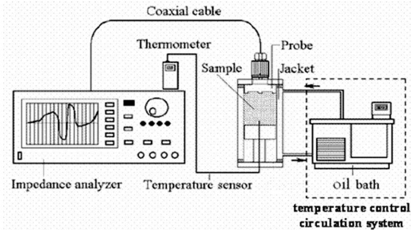
Fig. 1. Schematic diagram of the dielectric properties measurement system (Wang et al., 2005).
