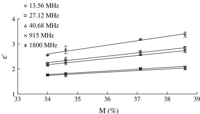
**Fig. 6.** Moisture content dependency of bread dielectric constant at five frequencies and 25 °C.
