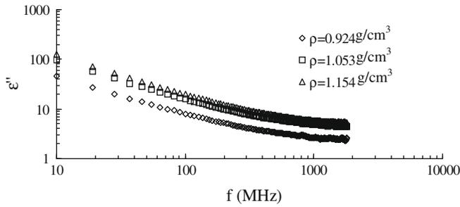
Fig. 3. Dielectric loss factors of compressed white bread samples with 37.1% moisture content at three densities and 23 °C.
