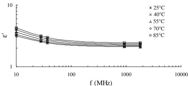
**Fig. 4.** Values of bread dielectric constant at five temperatures and 37.1% moisture content.
