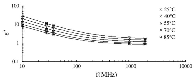
**Fig. 5.** Values of bread loss factor at five temperatures and 37.1% moisture content.
