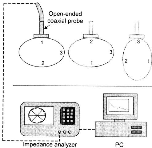
Figure 2. Measurement points on egg and experimental layout.
