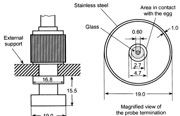
Figure 1. Schematic diagram of open-ended coaxial probe (all dimensions in mm).
