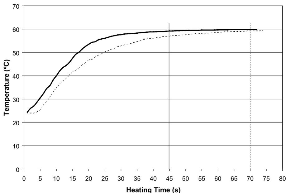
Fig. 2. A typical come-up time of liquid egg sample in a water bath at 60 °C. Solid line: Sample in a TDT disk; Dotted line: Sample in a glass tube (1 ml in 10 ml tube). The vertical lines represent the end of come-up time. The come-up time was determined when the center temperature of sample reached to 59.4 °C (99% of target temperature).
