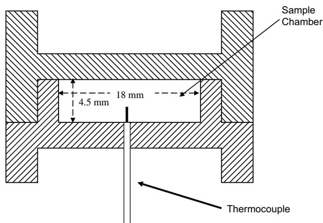
Fig. 1. Schematic diagram of aluminium TDT disk. Two halves are screwed together with an o-ring to provide a hermetic seal.
