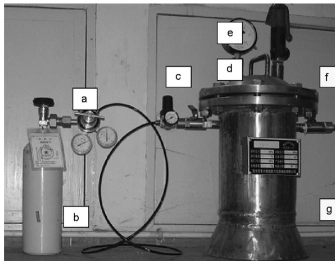
Fig. 1. Schematic diagram of apparatus to apply compressed Ar and Xe mix: (a) regulator, (b) mixed gas cylinder, (c) adjusting valve, (d) safety valve, (e) pressure gauge, (f) ball valve and (g) sample chamber.
