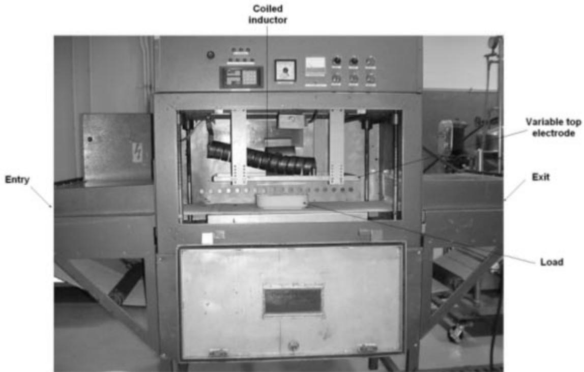
**FIGURE 1:** Front view of the 6 kW industrial RF parallel plate applicator (courtesy of Strayfield Ltd, UK).
