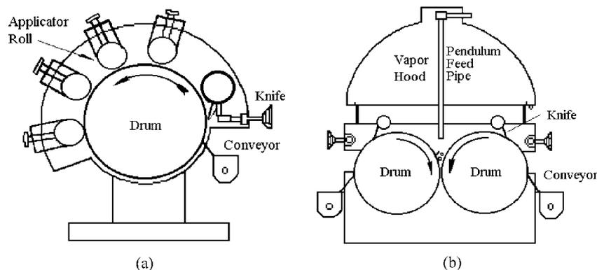
**Fig. 1** (a) Single drum dryer and (b) double drum dryer.
