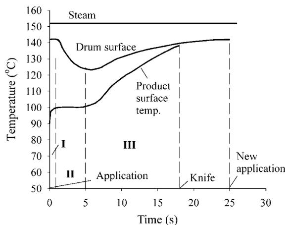
**Fig. 3** Product and drum surface temperatures during one revolution of drum drying in three different drying periods. (From Ref. 5.)
