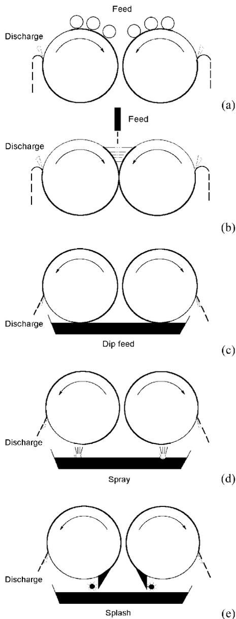
**Fig. 2** Feeding methods used in drum dryers: (a) roll feed; (b) nip feed; (c) dip feed; (d) spray; and (e) splash.
