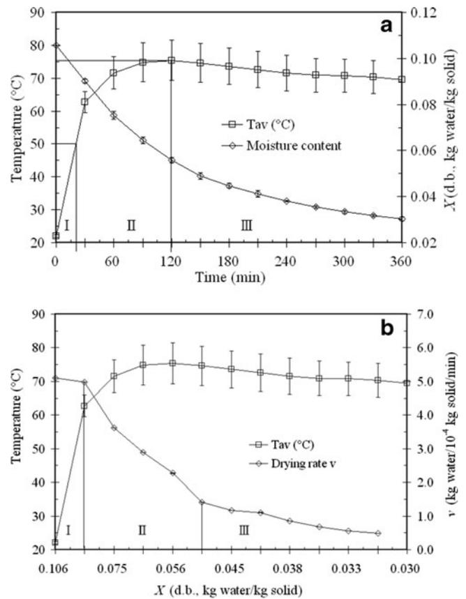
**Fig. 6** Drying curve (a) and rate (b) at three stages (I, II and III) with average sample surface temperatures ( $T_{av}$ ) measured by thermal imaging when subjected to hot air (50 °C) assisted radio frequency drying with an electrode gap of 15.5 cm
