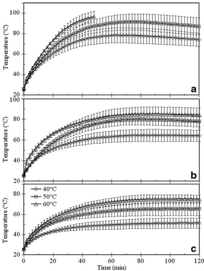
**Fig. 5** Average and standard deviation values of nut temperatures over seven locations with electrode gaps of 14.5 cm (a), 15.5 cm (b), and 16.5 cm (c) and when subjected to hot air (40, 50, and 60 °C) assisted radio frequency drying
