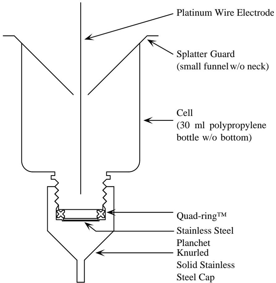
Fig. 1. Electrolytic cell.
