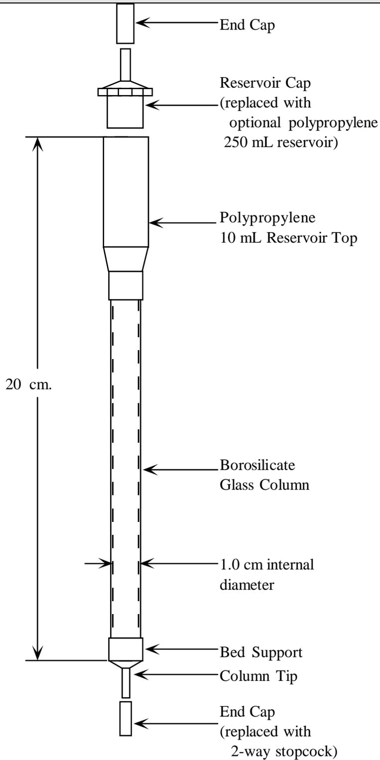
Figure 1. Ion Exchange Column
