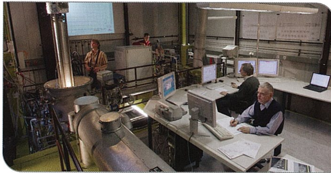
Quench experiments: In the Quench experimental facility, water is introduced into the superheated core of a light water reactor as a measure of temperature reduction.
