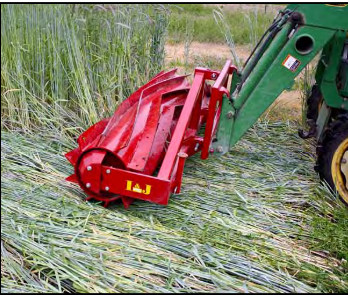
Roller/crimper mechanical termination.
