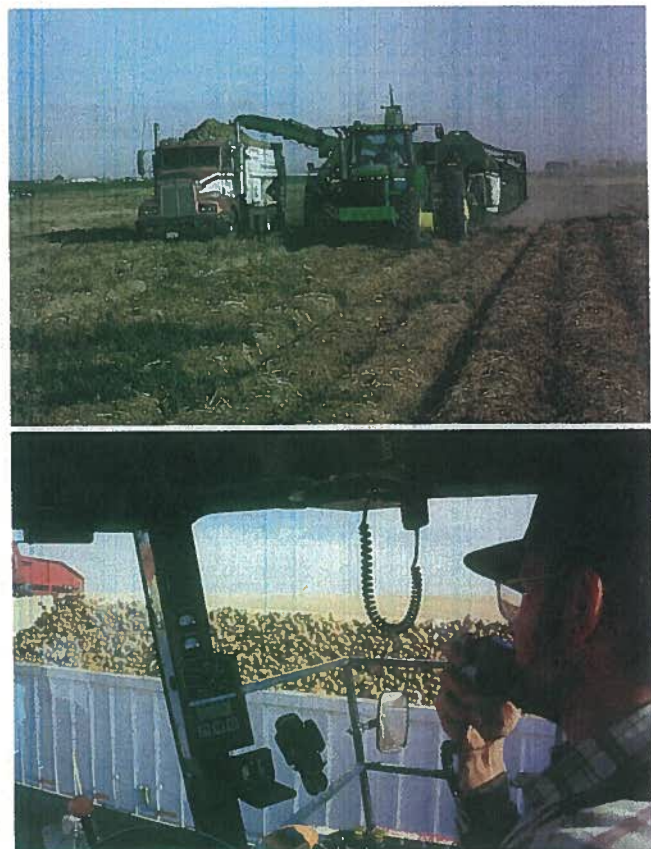
Fig. 10.5. Good coordination and communication between the harvester operator and the bulk truck operator are necessary to avoid dropping tubers into the truck from an excessive height or allowing the harvester's loading boom to plow into the pile of tubers on the truck. (Courtesy Washington State Potato Commission [top] and M. J. Pavek [bottom])
