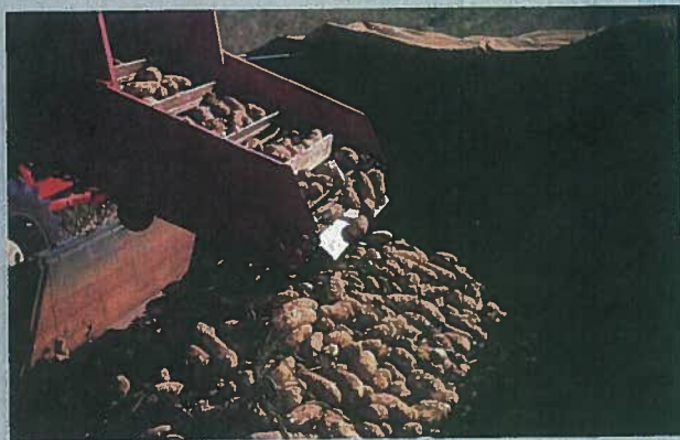
The drop from the conveyor should be limited to 6 inches.
