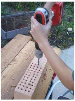
Drill out the intersections of the lines with a 5/16° drill bit, to a depth of about 3 inches. Do not drill all the way through the block. Photo by Jason Miller
