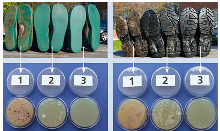
Figure 3. Demonstration of bacteria cultured from boots with smooth and patterned soles. 1 = dirty, 2 = washed with water, 3 = disinfected. Note that patterned-soled boots are more difficult to disinfect effectively and may still harbor bacteria. Photo courtesy of ILVO-UGent.
